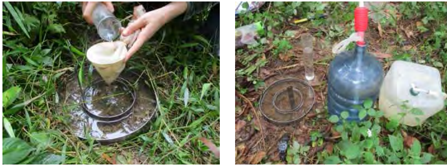
FIGURE 2.5: Application of the double-ring infiltrometer. Water was pumped from water gallons into the measuring cylinder (right) and from there poured into the inner ring (left) while the outer ring was filled directly with the pump.
