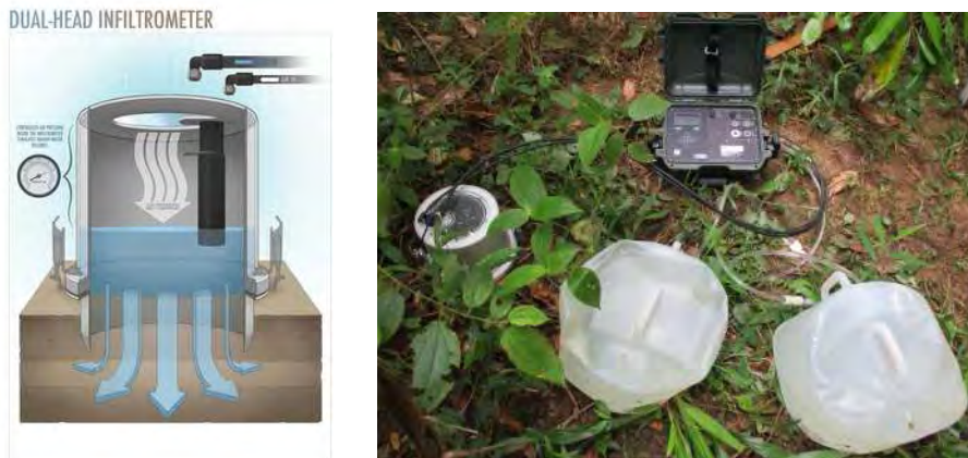
FIGURE 2.4: Application of the dual-head pressure infiltrometer. Left: Set-up with control unit, water tanks and infiltrometer head. Right: Functionality with water and air inputs and the pressure sensor (METER Group, 2017b).
